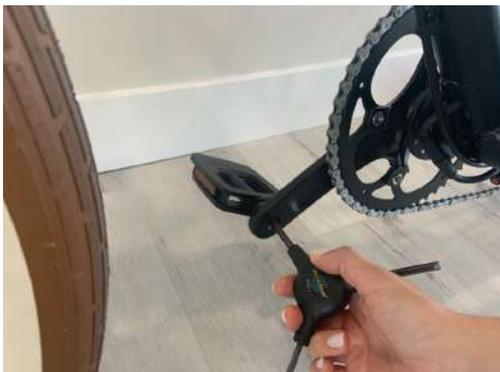
Begin the installation by twisting the pedal into the correct pedal arm by hand. Once the pedal becomes too difficult to twist by hand, further tighten with an M6 hex wrench.
