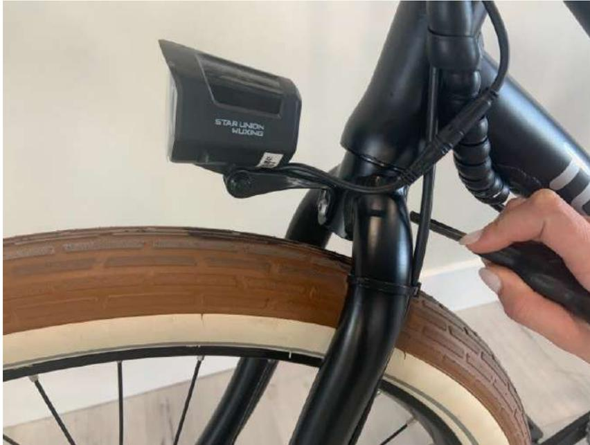
Tighten using a crescent wrench and a M4 hex wrench to ensure a secure fit. There will be a cable with a red connector dangling from the wiring harness near the head tube. Connect your headlight cable to this red connector, ensuring you very carefully align all three prongs. Make sure the cable is routed on the side to allow movement of the forks.
