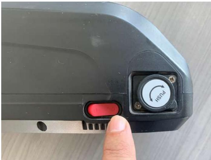
To remove the battery, rotate the key counterclockwise to unlock the battery from the controller dock. It is not removable when locked. Use one hand at the bottom of the battery to lift it from the base position of the dock upwards. Pull the battery upwards and away from the dock, then remove it by lowering it out and back down and tilting the bottom to the left and out to clear the rear frame triangle.
