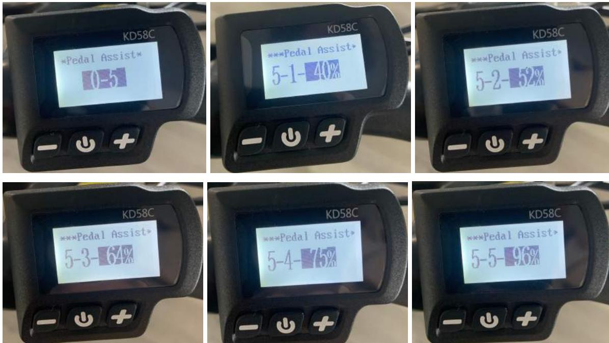
After the desired PAS ratio for each power level is input for all 5 pedal assist levels, press the **POWER** button to confirm and return to the advanced settings interface.
